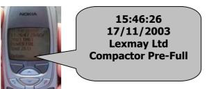
status of a machine. Each individual Waste Watcher can be configured (by the host terminal) so that some or all of its status events are forwarded to, up to 3 individual phone numbers
